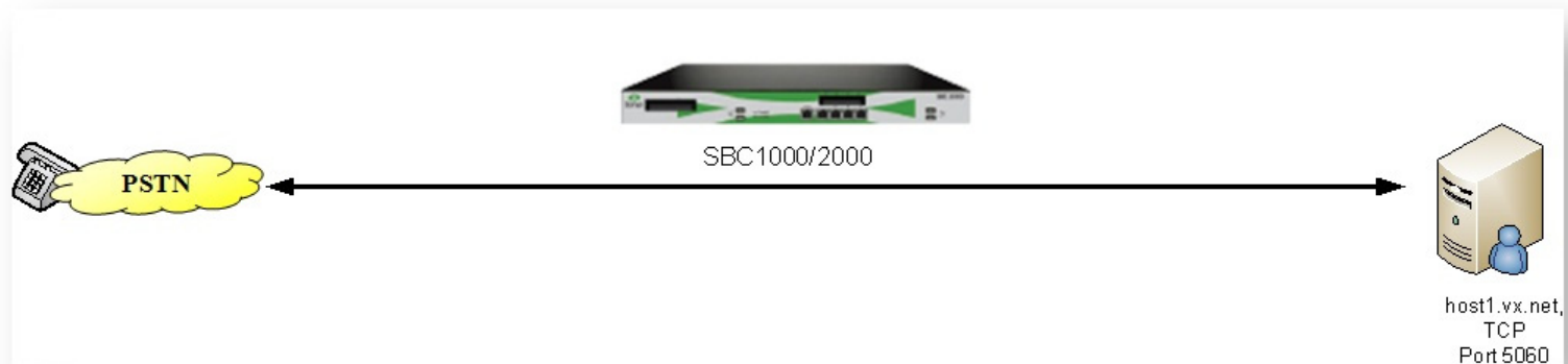
ISDN to SIP (TCP) Network
